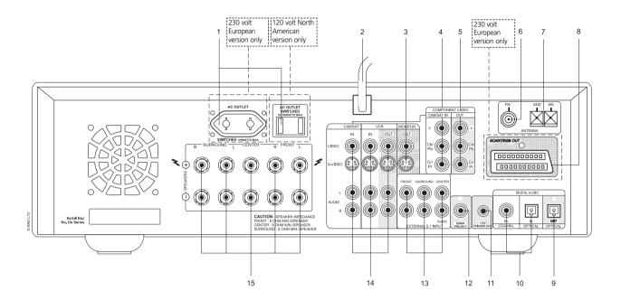
SWITCHED AC OUTLET: This convenience jack can supply switched power to another component or accessory. It is powered on and off by the front panel POWER key (or the HTR L73's ON and OFF keys).
